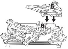
Figure 45 - Installing Logs No. 5 and No. 6
